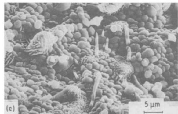
Figure 2 SEM fractographs of sintered samples after thermal quench cycles between 1150 °C and water at 25 °C (RT). (a) M_{10} (42 cycles—F); (b) M_{10}T_4 (50 cycles—NF); (c) M_{10}T_6 (50 cycles—NF); F, failed; NF, not failed.
