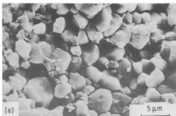
Figure 2 SEM fractographs of sintered samples after thermal quench cycles between 1150 °C and water at 25 °C (RT). (a) M_{10} (42 cycles—F); (b) M_{10}T_4 (50 cycles—NF); (c) M_{10}T_6 (50 cycles—NF); F, failed; NF, not failed.
